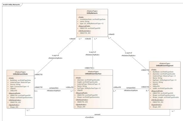
Figure 6. The logical data model of utility networks.
