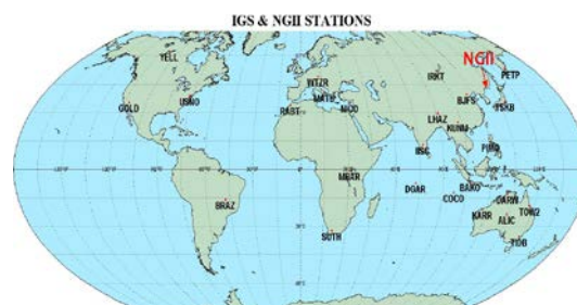
Figure 4. Selected IGS station and location of NGII GPS network in Korean Peninsula.
