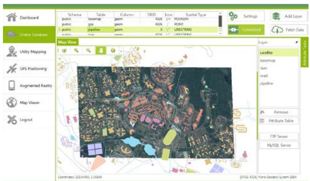
Figure 5. The mobile mapping application main interface shows raster layer (satellite) being mapped collaboratively with others layers using data from database.gpkg.
