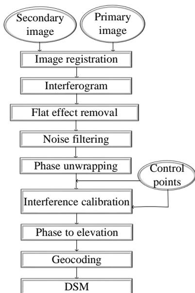
Figure 2. The flow chart of generation DSM using airborne InSAR data
