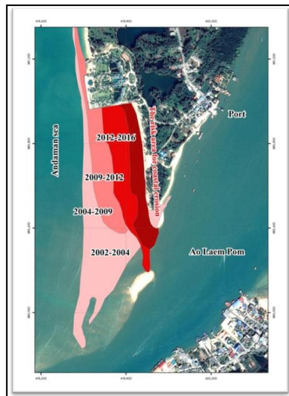
Figure 5. The severe erosion of Koh Kho Khao and the special monitoring area
