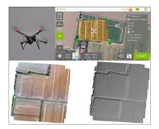
Figure 7. Elements of Drone Survey. From top left clockwise – Drone Phantom 4 DJI, flight plan with parameters, DSM hillshade and orthophoto 2cm GSD.
