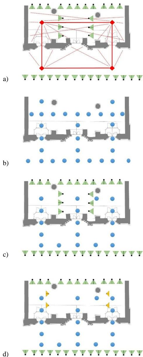
Figure 1. Some configurations for the survey of interior and exterior spaces: (a) total station (red diamonds) + central perspectives images (green triangles), (b) 360° images (circles), (c) 360° + central perspectives images, (d) 360° + central perspectives + fisheye images (yellow triangles).
