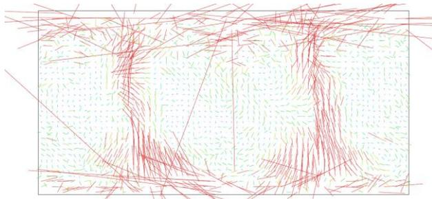
Figure 4. Image coordinates residual after bundle adjustment. A systematic effect in the overlapping area between front- and rear-facing images is clearly visible.
