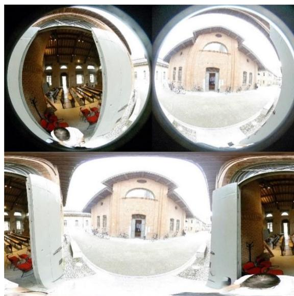
Figure 3. The original images acquired from front- and rear-facing cameras (top) and the final spherical image generated by stitching the previous images (bottom).
