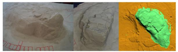
Figure 3. The historic physical 3D model of the Kalkberg (left), the historic digital 3D model from dense image matching (centre) and the combination of two DEMs from both today (orange) and the past (green) (right)
