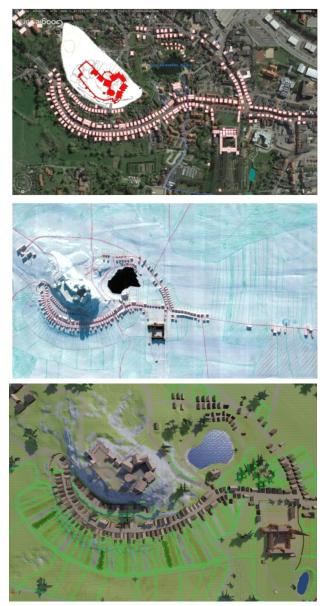
Figure 8. Aerial orthophoto superimposed with historic buildings (top), raw 3D model with landscape and property sketch (centre), and textured 3D model in the Unreal Game Engine (bottom, green lines represent fences for property areas). For better comparison with the engraving, south is up.
