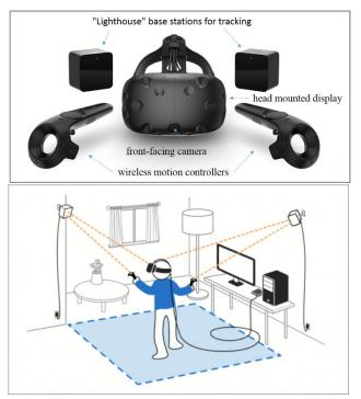
Figure 9. The components of the VR System HTC Vive (top) and system setup of the HTC Vive (bottom) (HTC Corporation 2017)
