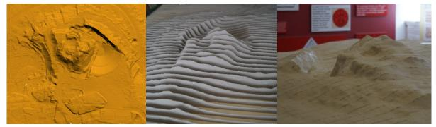
Figure 2. The reconstruction of the Kalkberg from airborne laser scanning data: digital elevation model (original data, left), printed scaled sections of the DEM (centre) and physical 3D model of the Kalkberg at it exists today (right)
