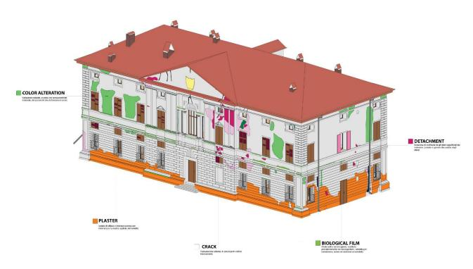
Figure 15. 3D visualization of the parametric model of Villa Sarmoris with the mapped decay.
