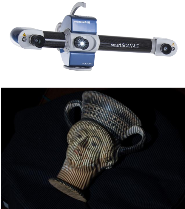
Figure 2. SmartScanHE C8 fringe projection scanner (above). Fringe projection scanning process on attic head vase (below, Antikensammlung Berlin).
