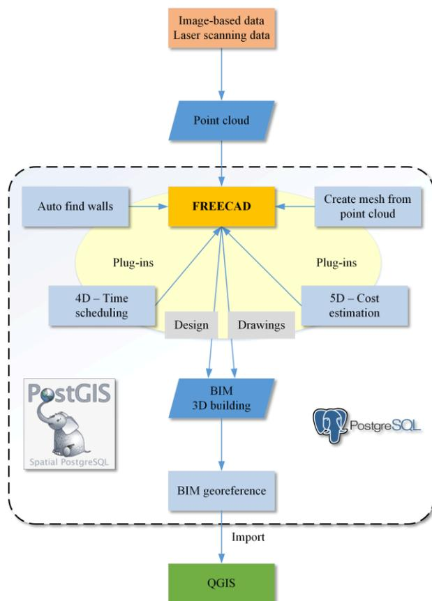
Figure 1: BIM ecosystem around FreeCAD
