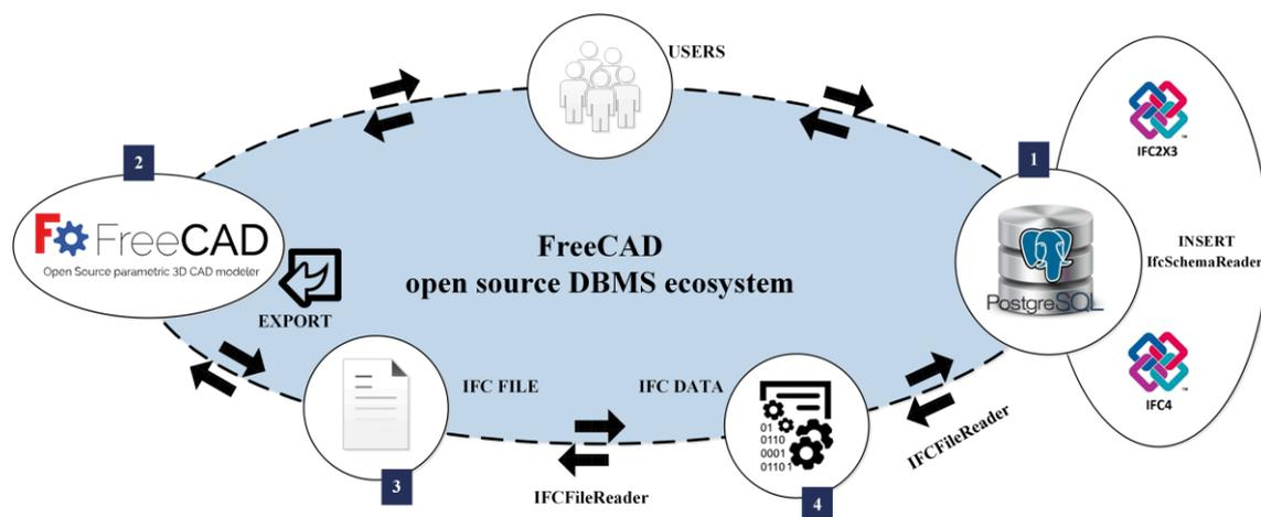
Figure 6: Workflow chart for FreeCAD open source DBMS ecosystem
