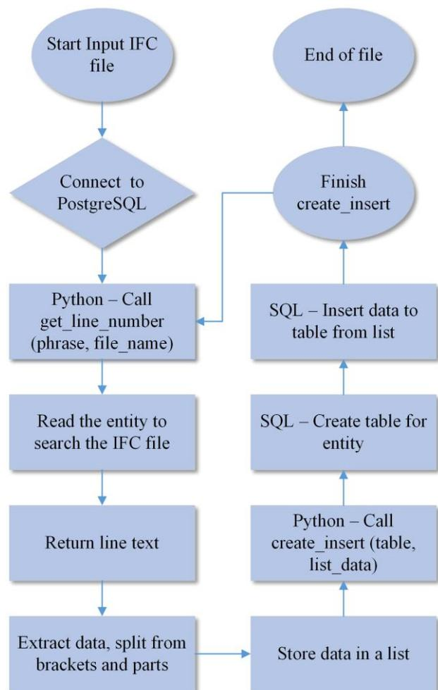
Figure 9: Diagram that shows the store method of IFC data in PostgreSQL
