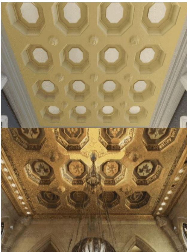
Figure 2. Screenshots from the Senate chamber ceiling animation: the BIM animation made with Enscape (top), and the point cloud animation made with Pointools (bottom)
