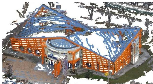
Figure 5. The „Dean’s office” building model created in the Visual SfM software based on UAS images, represented as a point cloud
