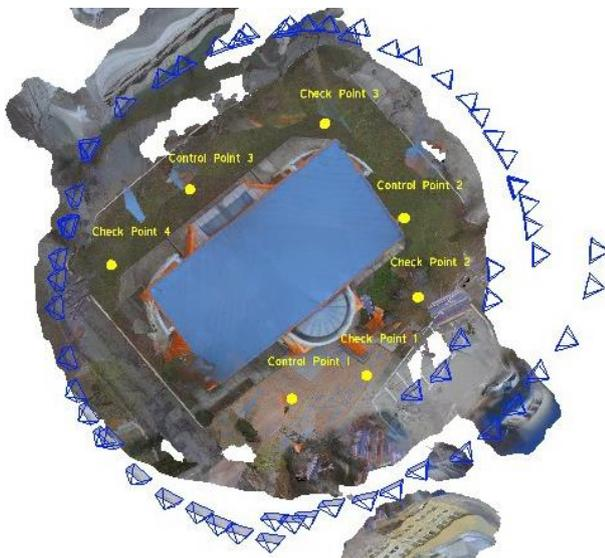
Figure 4. The visualization of the Control Points 1, 2 and 3, the Artificial Check points 1, 2, 3 and 4 and the camera positions and orientations
