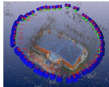
Figure 6. The camera positions and orientations and the dense point cloud
