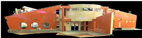
Figure 1. The TLS point cloud with realistic colour information
