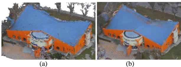
Figure 8. The „Dean’s office” building model, created in the Drone2Map software based on UAS images point cloud (a), mesh surface (b)
