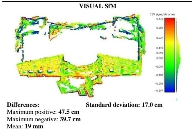
Figure 11. The residuals of the facades UAS point clouds obtained by using different software
