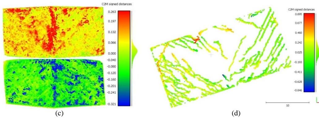
Figure 10. The Hausdorff distances calculated for the roof UAS point clouds obtained by different software: Zephyr (a), PhotoModeler Scanner (b), Drones2Map (top view and bottom up view) (c) and Visual SfM (d), using as reference data the mesh created based on GNSS measurements
