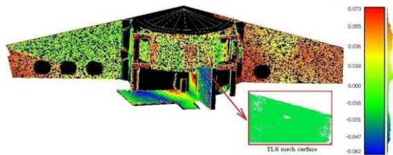
Figure 12. The Hausdorff distances calculated for the sample points generated for the front facade
