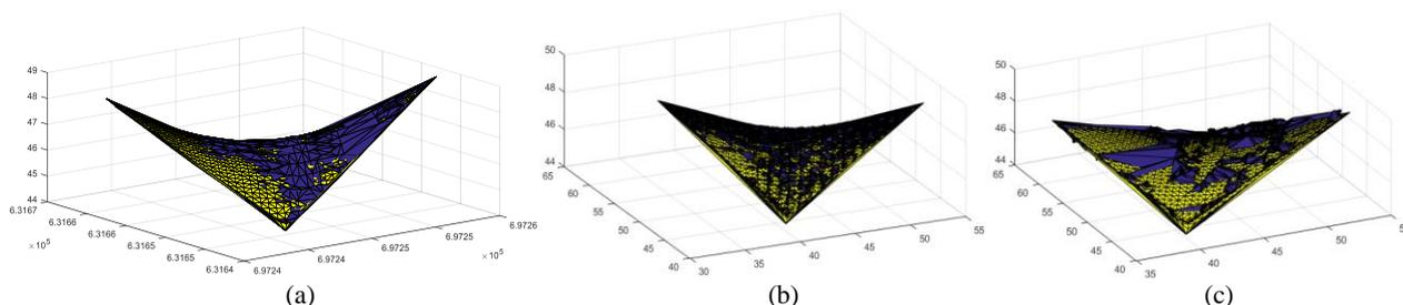
Figure 9. The roof surface modelled in 3D (blue colour) using the GNSS points (a) , Zephyr point cloud (b), Visual SfM point cloud (c) and the best fitting hyperbolic paraboloid shape (yellow colour) from the east side
