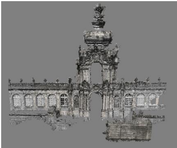
Figure 3. Point cloud generated from historical images (exterior view of the Zwinger)
