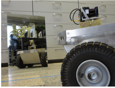
Figure 1: Robot equipped with the 3D-Hokuyo multi-echo laser scanner facing an unframed mirror.
