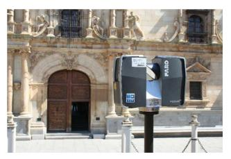
Figure 8: Picture of the laser scanner FARO FOCUS 120 and the San Ildefonso College Facade.
