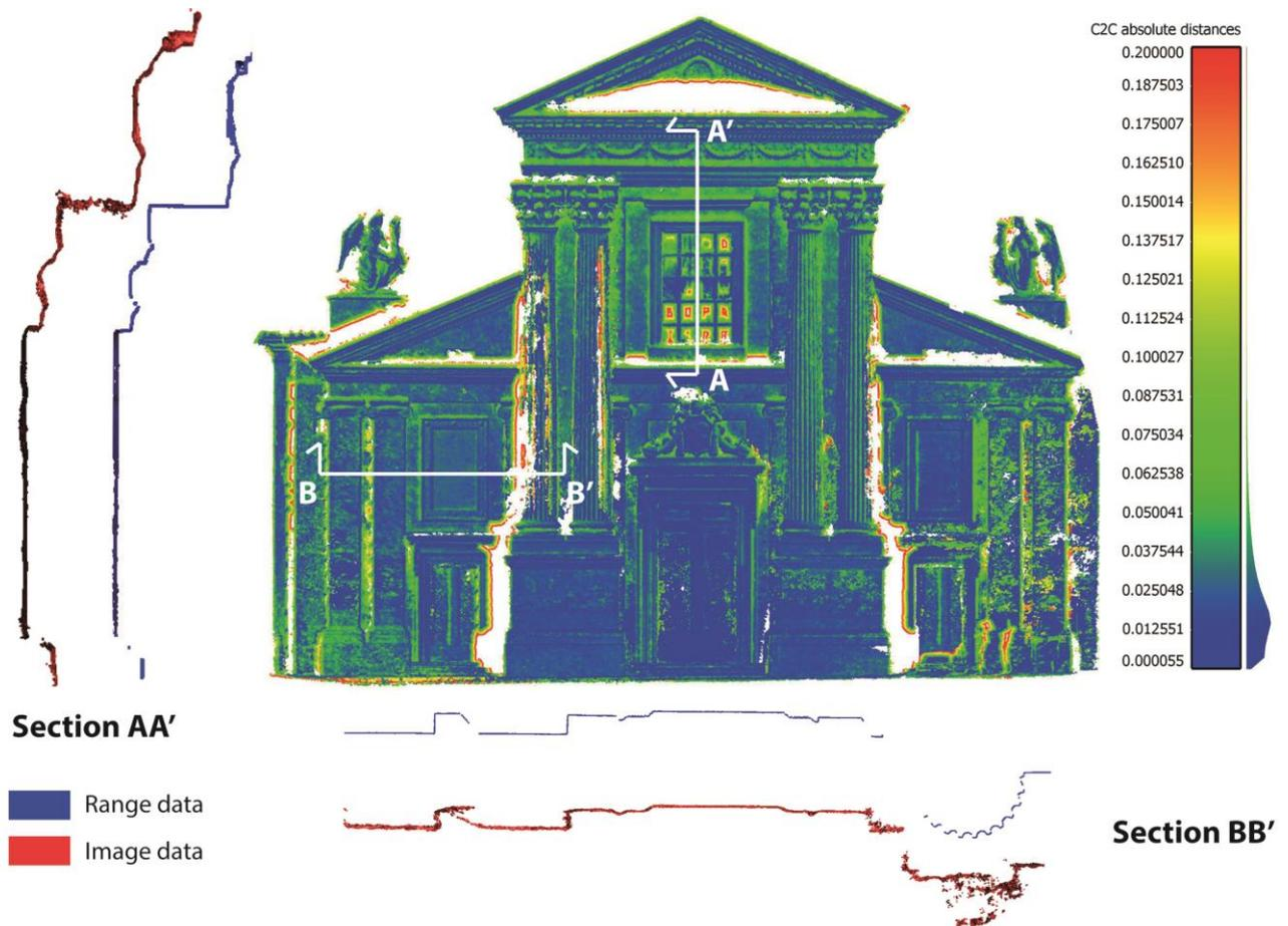
Figure 7. Deviation map between the photogrammetric cloud and range data, with two relative sections.
