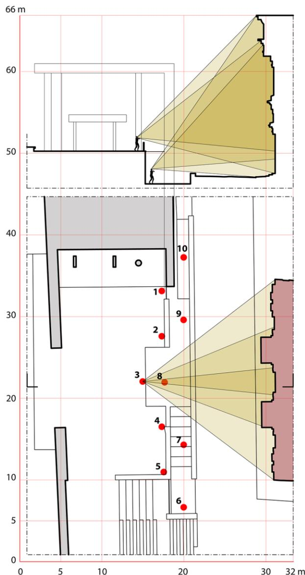
Figure 4. Photogrammetric survey schema. The plan shows the cameras acquisition network and the horizontal image rotation from point of view #3; in section a pair of acquisition points whit vertical baseline and rotation with 2 images.
