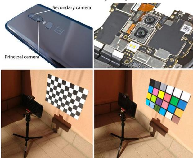
Figure 2. Above the external and internal back view of the A6000 (OnePlus) smartphone, below two testing phases of the smartphone camera with b/w and coloured targets.
