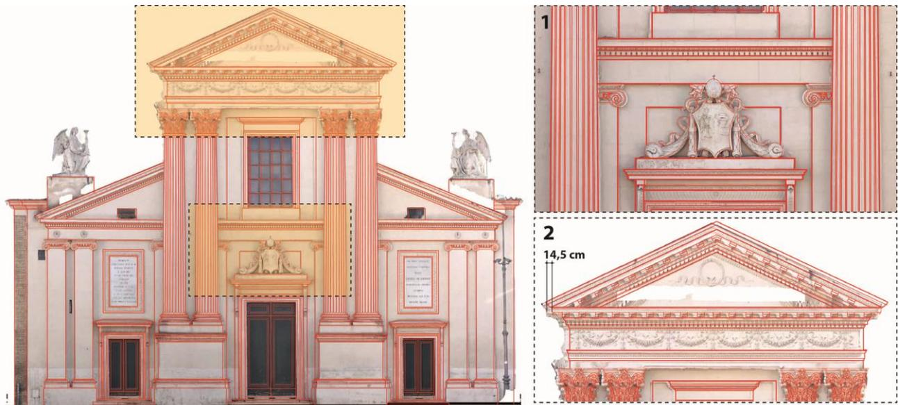
Figure 8. Overlapping of the façade drawing with the orthophoto, with close-up on two specific areas.
