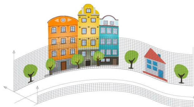
Figure 4. The coordinate system of the road with the corresponding grids of the left and right side
