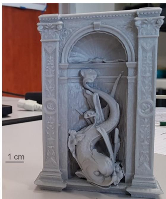
Figure 10. Example of 3D printed fish (on the left side of the fountain)
