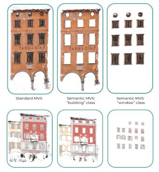
Figure 6: Dense point cloud of a building façade using the standard patch-based MVS algorithm as implemented by OpenMVS (left) and after applying the proposed semantic constraints keeping only points under "building" (middle) and "window" (right) classes. Noisy and undesired 3D points under label "obstacle" or "sky" are automatically excluded.
