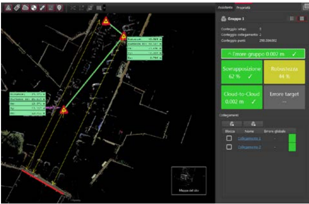
Figure 5. TLS survey processing information
