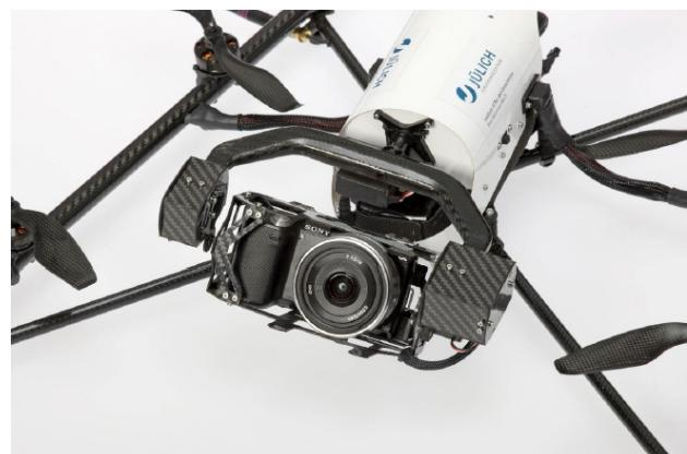
Figure 3. Sony Alpha 6000 camera attached to the Falcon-8 Octocopter.
