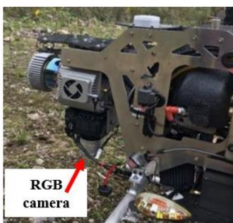
Figure 4. RGB camera mounted on UAV in 2018 flight campaign
