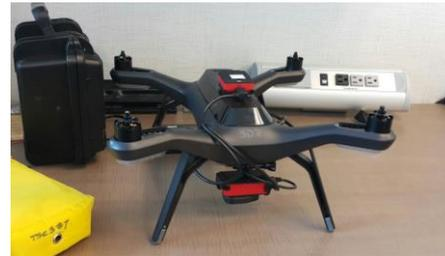
Figure 7. 3DR Solo UAV equipped with the Sequoia Imagery Sensor.
