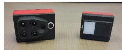
(a): The Sequoia camera on the left, while the GPS /IMU sensor on the right.
