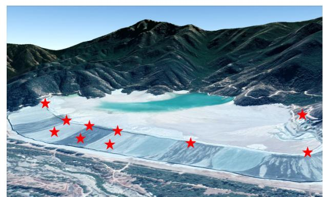
Figure 6. Planned positions (red asterisks) of 10 GNSS devices. 5 corner reflectors will be integrated to five of these positions (under discussion).
