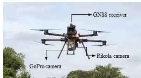
Figure 2. UX4 UAV and its payload
