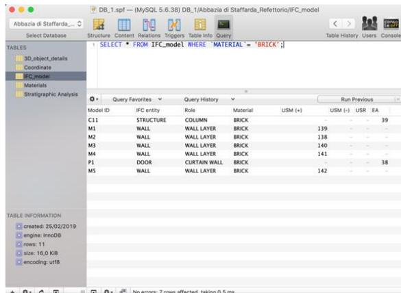
Figure 5. DBMS concerning IFC objects and stratigraphy
