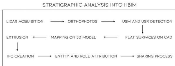
Figure 3. From stratigraphic analysis to IFC models
