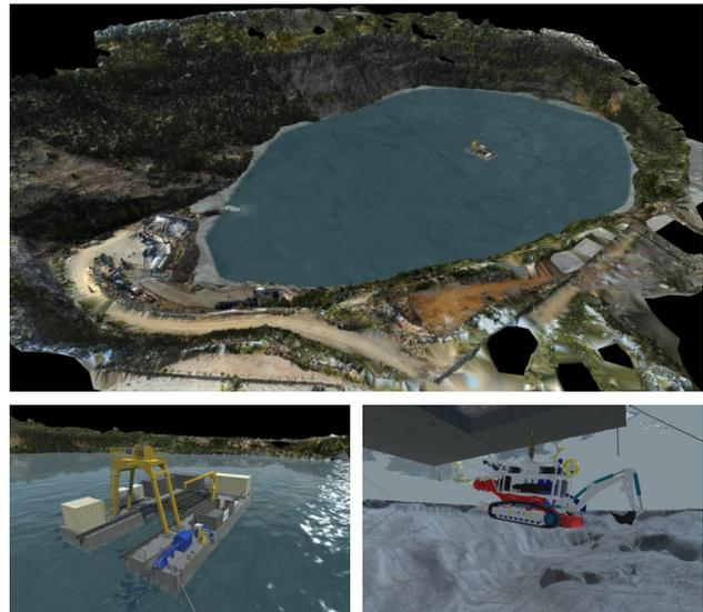
Figure 5. Model of the mining site in VR. Top: model of the mine with colored mesh of the above-the-water terrain, bottom: detail view of the launch and recovery vessel and the mining vehicle with underwater terrain model.
