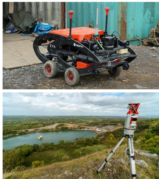
Figure 4. Equipment used for the above-the-water and underwater survey of the mine site. Top: the EVA AUV/HROV used for the multibeam sonar survey of the mine, bottom: survey of the Silvermines mine site using terrestrial laserscanning.
