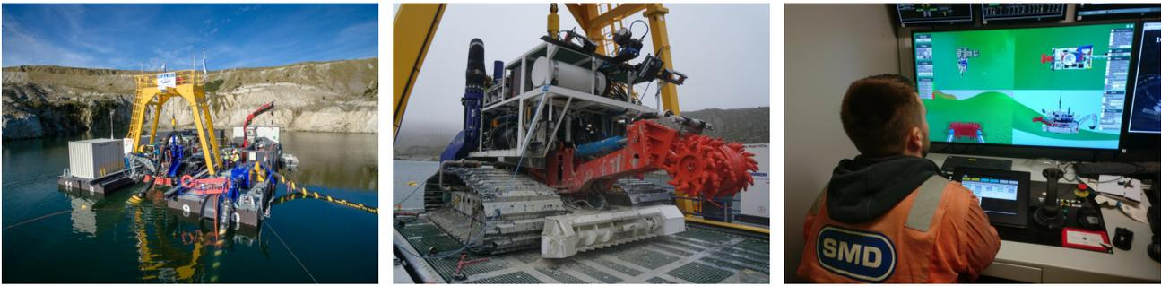
Figure 2. iVAMOS! underwater mining system. Left: launch and recovery vessel during deployment of the mining vehicle, middle: iVAMOS! mining vehicle with roadheader cutting machine and perception sensors, right: tele-operation of the mining vehicle using the VR based human-machine interface.
