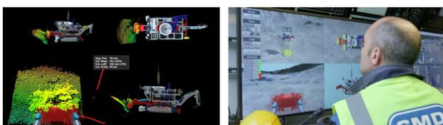
Figure 7. Split-views for piloting the mining vehicle during cutting operations. The view point for each split view can be adjusted individually.
