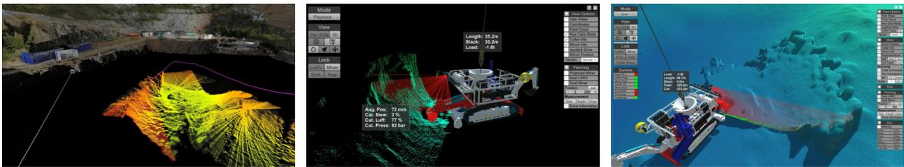
Figure 6. Different views of the VR based human-machine interface. Left: live multibeam data visualization during a survey using the EVA AUV/HROV, middle: mining vehicle with visualization of multibeam sonar scans, right: mining vehicle with updating terrain model using a mechanically panning multibeam sonar.
