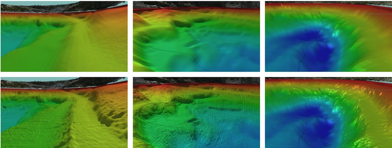
Figure 8. Bathymetry of the Silvermines flooded opencast mine. Top: pre-survey created by a surveyor, bottom: updated survey created using multibeam sonar.
