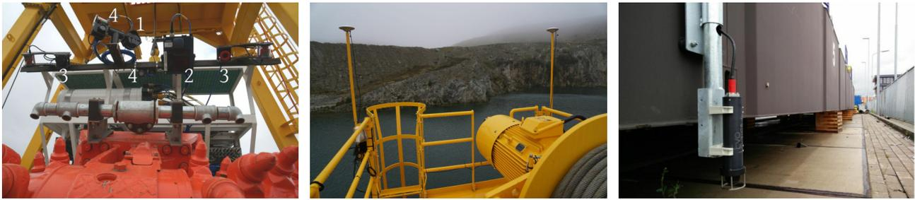
Figure 3. Perception and positioning sensors. Left: perception sensors mounted to the sensor bar on the front of the mining vehicle, middle: GNSS antennas mounted on the top of the launch and recover vessel, right: SBL acoustic transponder mounted on the corners of the vessel for underwater positioning.
