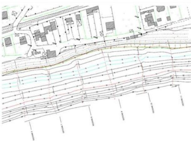
Figure 10. Echosounder bathymetry
