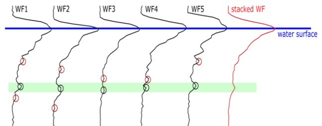
Figure 6: Basic principle of waveform stacking applied to ALB pulse echo waveforms (Mader et al., 2019)
