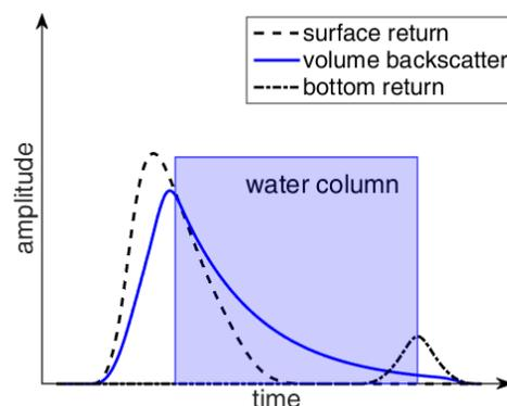
Figure 1: Waveform of a prototype ALB laser pulse echo (Richter et al., 2017)
