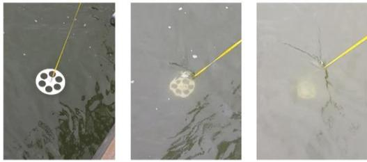
Figure 8: Estimation of visibility depth by lowering a Secchi-disk into the water body
