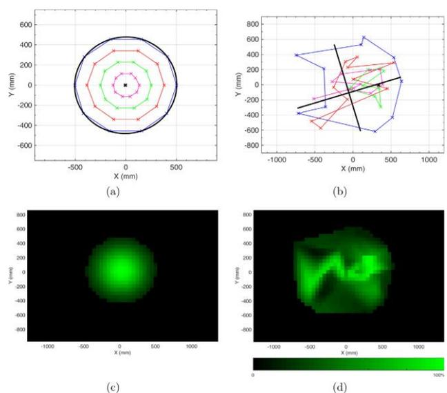
Figure 4: Wave-induced changes in laser spot size and shape on a simulated wave pattern – left water surface, right water bottom (Westfeld et al., 2017)
