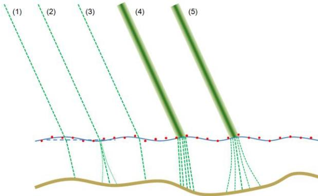
Figure 2: Different representations of the laser beam – water surface interaction (Westfeld et al., 2017)
