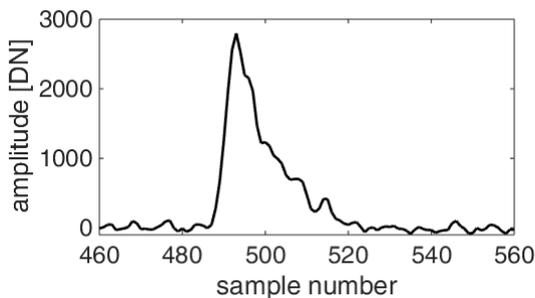
Figure 5: Example of a digitized waveform with poor bottom point echo recognizability (Richter et al., 2017)
