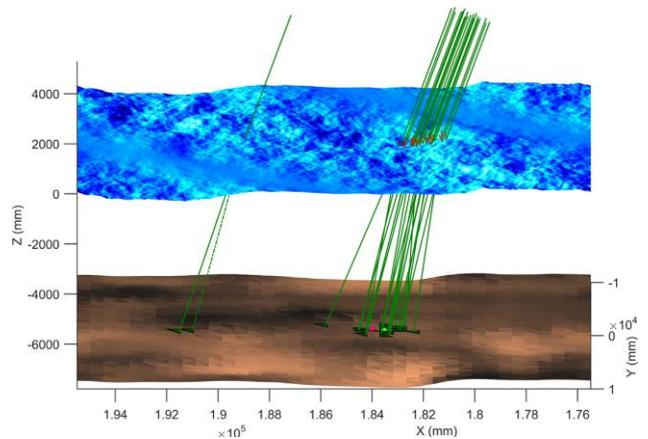
Figure 3: Interaction of an infinitesimally thin (left) and a finite diameter laser pulse (right) with a simulated wave pattern, effects on bottom point determination (Westfeld et al., 2017)
