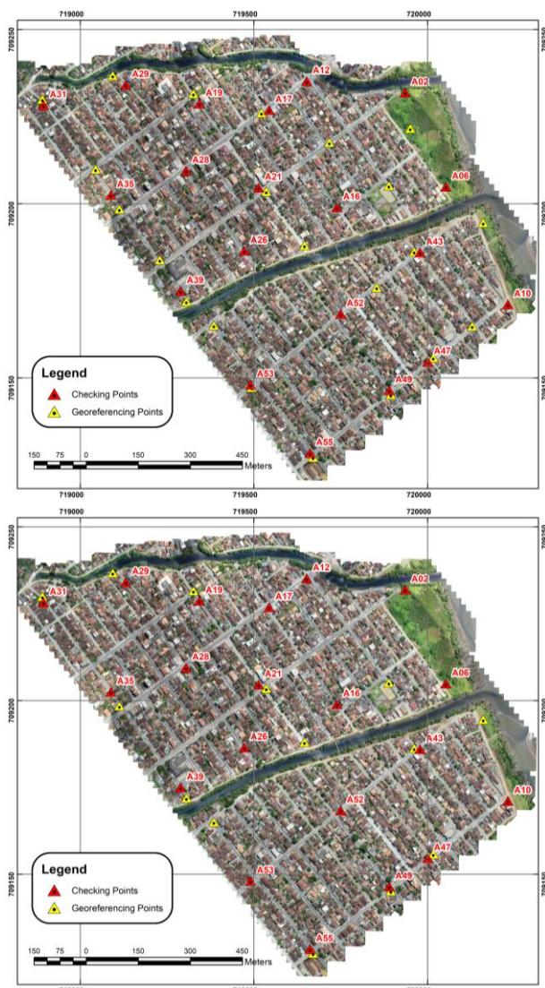
Figure 4. Orthophoto of the 1,0 km<sup>2</sup> area surveyed georeferenced with 30 and 20 GCPs and checking points used for the measurement of the RMSE
