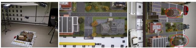
Figure 1. The test-object and acquisition scenario adopted for the *3DOMcity* photogrammetric contest: setup for data collection (left) and examples of nadir (centre) and oblique (right) images. Red ellipses highlight the buildings selected for DIM evaluation.
