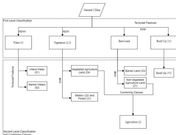
Figure 2. Flowchart of the applied classification methodology.
