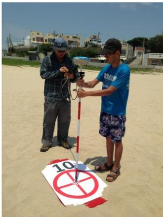
Figure 3. We used VRS system to survey the 18 GCPs
