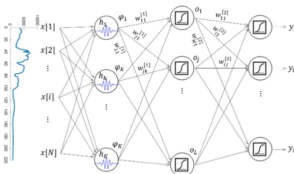
Figure 2. The structure of wavelet networks
