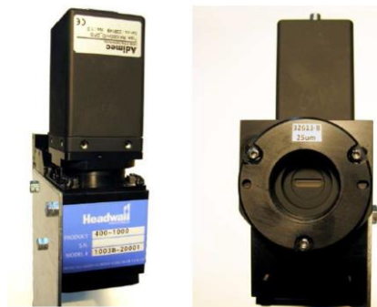
Figure 1. The push-broom hyperspectral imager- the Headwall MicroHyperspec A-series VNIR
