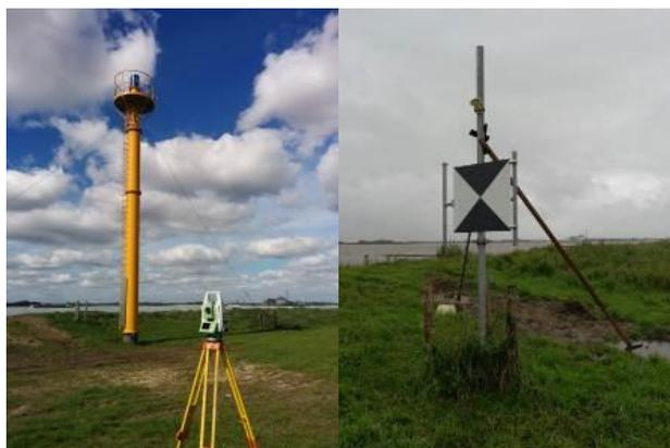
Figure 3. Platform for monitoring system at the bottom of the summer dyke (left), strutted pile with reference target as chess pattern 80x80 cm<sup>2</sup> (right)
