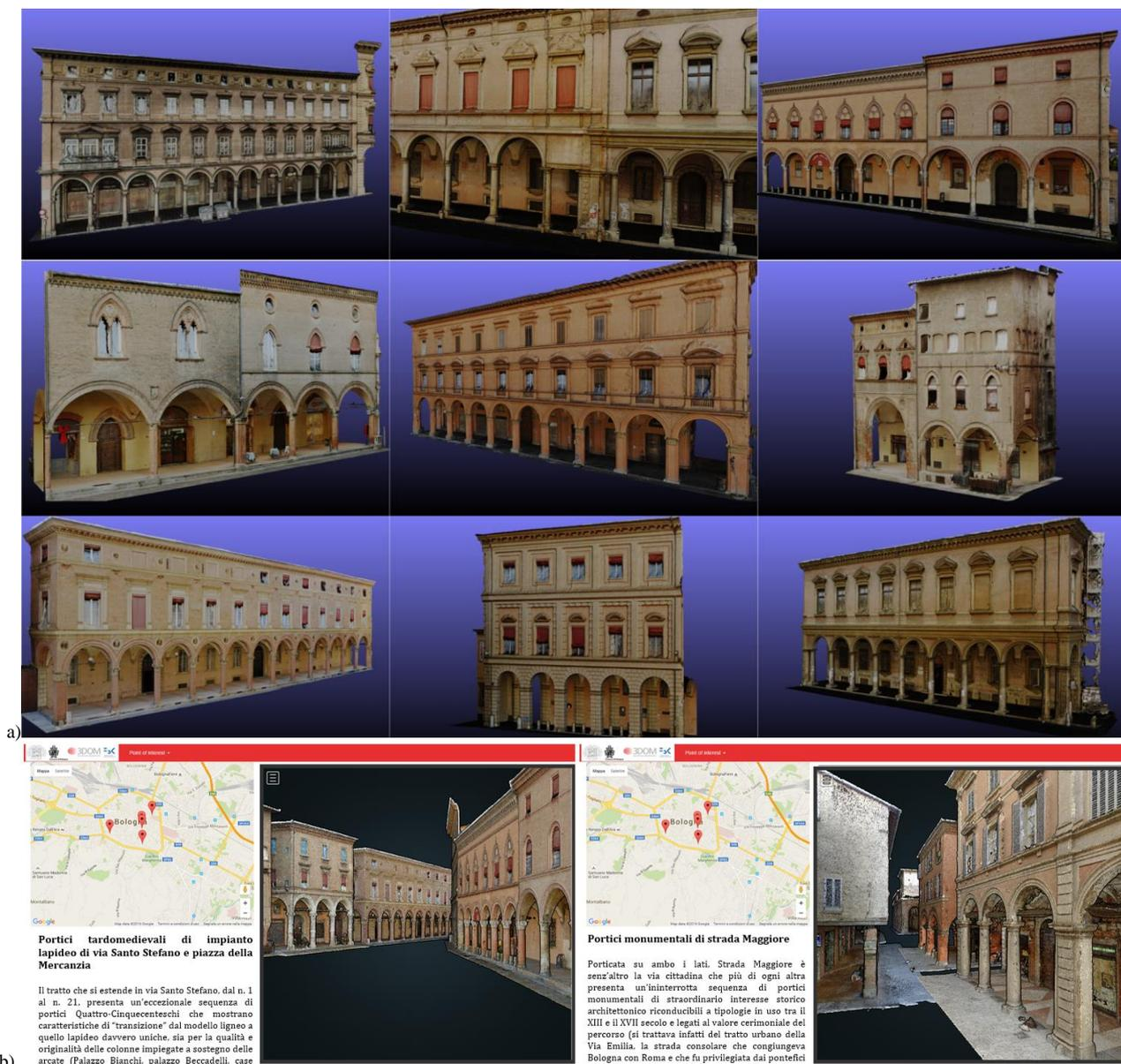
Figure 8: Examples of porticoes digitized using the presented methodology, shown as mesh models (a) and inside the point-based web viewer (c).
