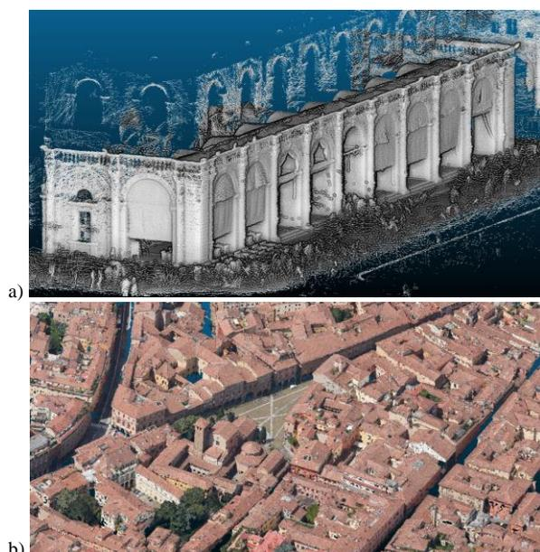
Figure 3: Examples of 3D reconstructions achieved with the evaluated sensors and techniques: portable/handheld 3D scanning (a) and oblique aerial images (b).
