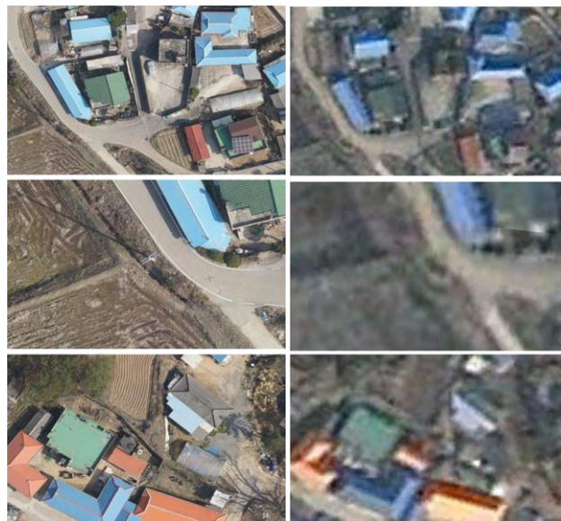
Figure 9. Orthoimages produced by our software (left) and served by Google Earth (right)
