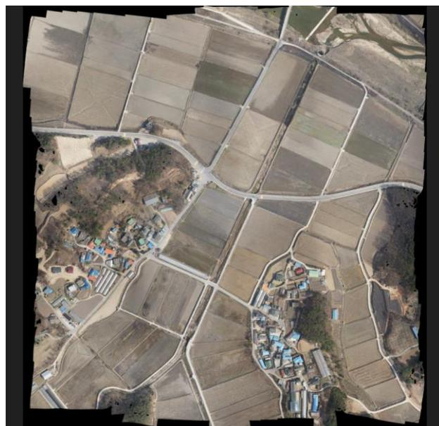
Figure 10. Orthoimage mosaic (flight altitude: 200 m)
