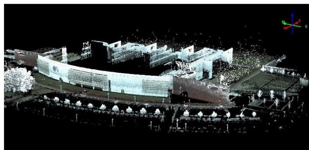
Figure 3. OS Explorer House point cloud captured using a Leica Pegasus backpack
