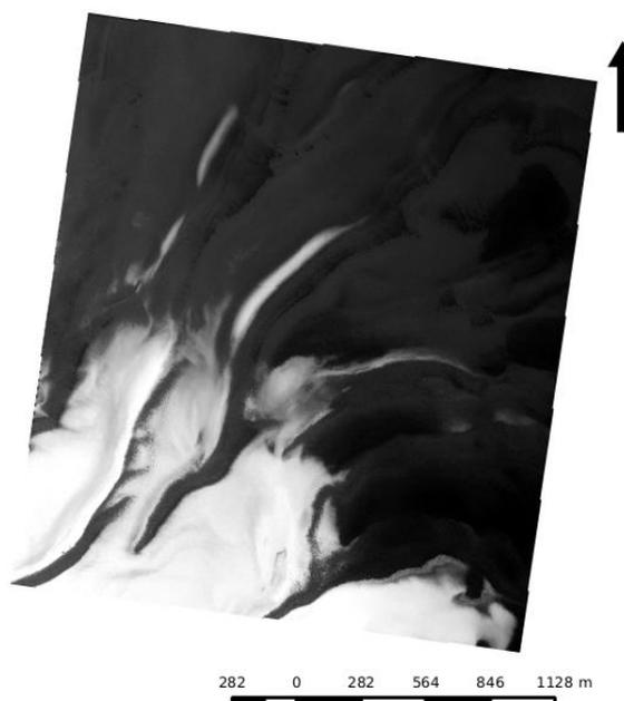
Figure 3. HRSC Image h2162\_0000, lines 1-15000 processed with DLR-VICAR, orthorectified to a DTM produced with the Kim & Muller (2009) Modification
