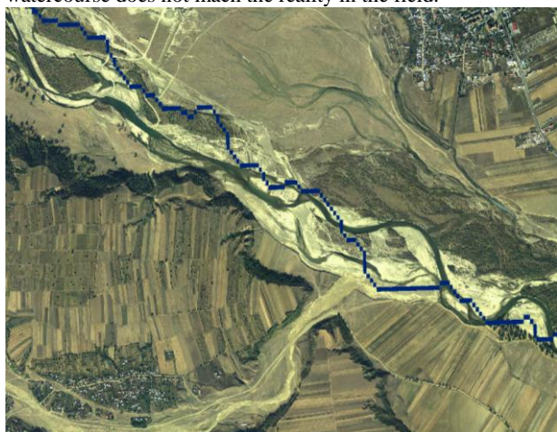
Figure 3. Obvious differences between the real path of the watercourse and the 30m SRTM delineated course
