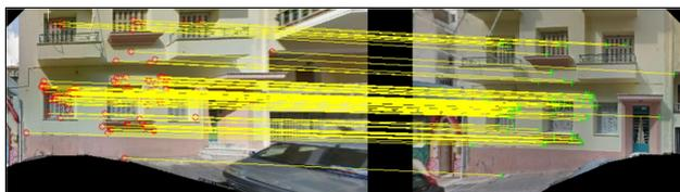
Figure 10. Tentative matches obtained by the ASIFT operator.
