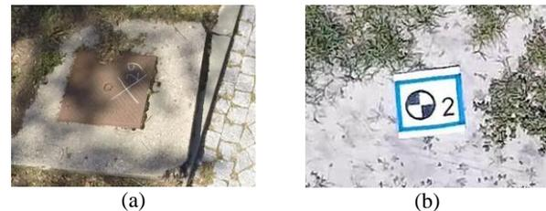
Figure 2. Images of the types of points used: (a) point marked with chalk and (b) signals.
