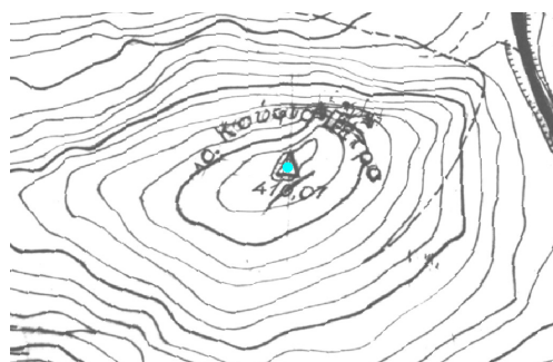
Figure 4. A trigonometric point on the map which is used as CP.
