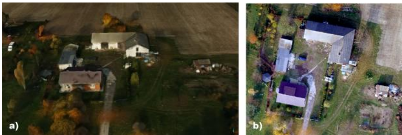
Figure. 3. Example of a) 3D mesh from dense-image-matching point cloud and b) part of the true-ortho
