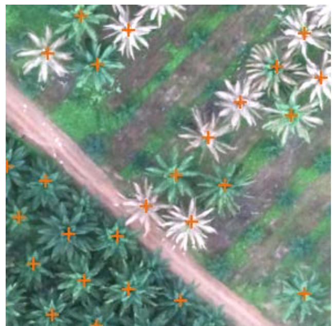
Figure 6: Results of tree detection (orange crosses) using a template matching algorithm that was populated with templates of oil palm trees.
