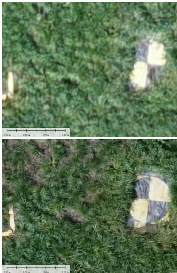
Figure 5: Demonstration of different GSDs (top: 2.4 cm, bottom: 1 cm).
