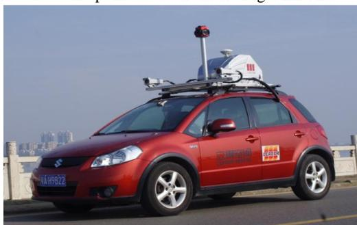
Figure 6. The mobile measure car
