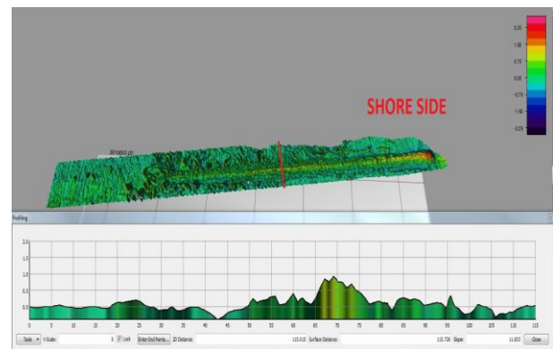
Figure 16: Change detection profile of the middle of the channel.
