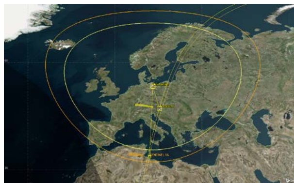
Figure 1. Ground Station Neustrelitz, acquisition circle for Sentinel-1 and TerraSAR-X; 5 degree elevation
